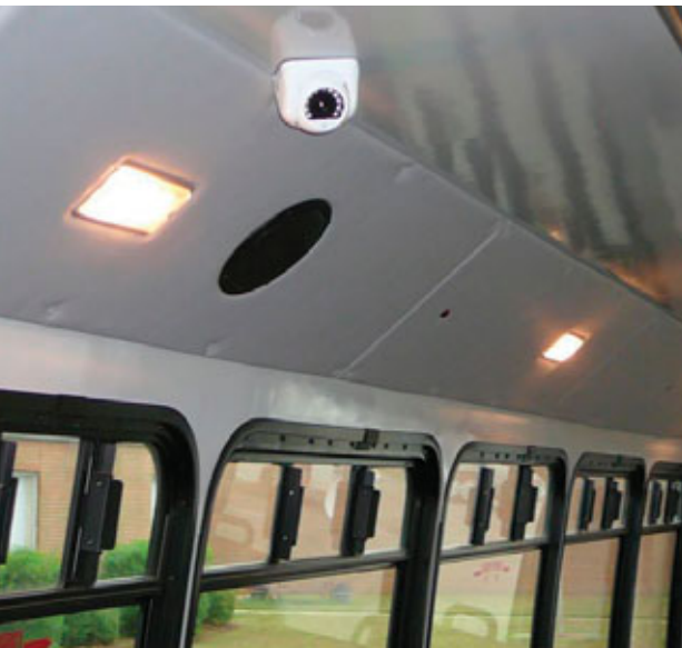
The AngelTrax TR2100, with built-in vandal-proof cast housing, is pointed toward the front of the bus and films the driver and entry well.
