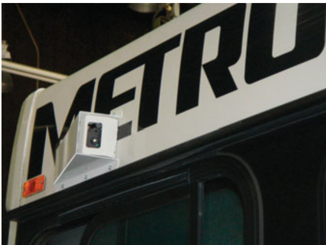
The Safety Vision SV-640 exterior wedge camera, placed on the side of a transit bus, can be used to monitor exits or to view surrounding traffic.
