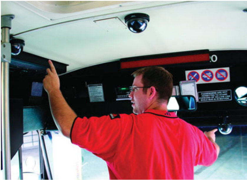
Dome cameras, such as this REI model, are prevalent in vehicles because they are tamper resistant.
